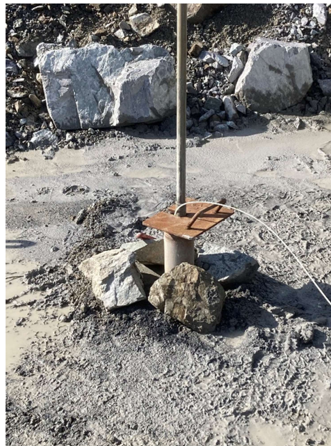
Photo 6: Packer test in AE22-MW104
